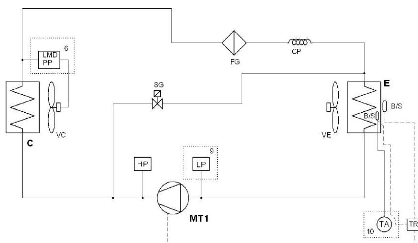
The compressor (MT1) compresses the coolant gas, taking it to a high pressure and temperature;
