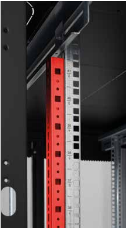
■ Vertical rails strengthening member Additional profile that increase vertical rails stability (4 pcs). It increase cabinet max. load to 1500 kg.
