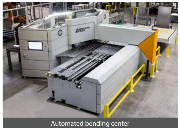
Metal forming line of skeleton rails
