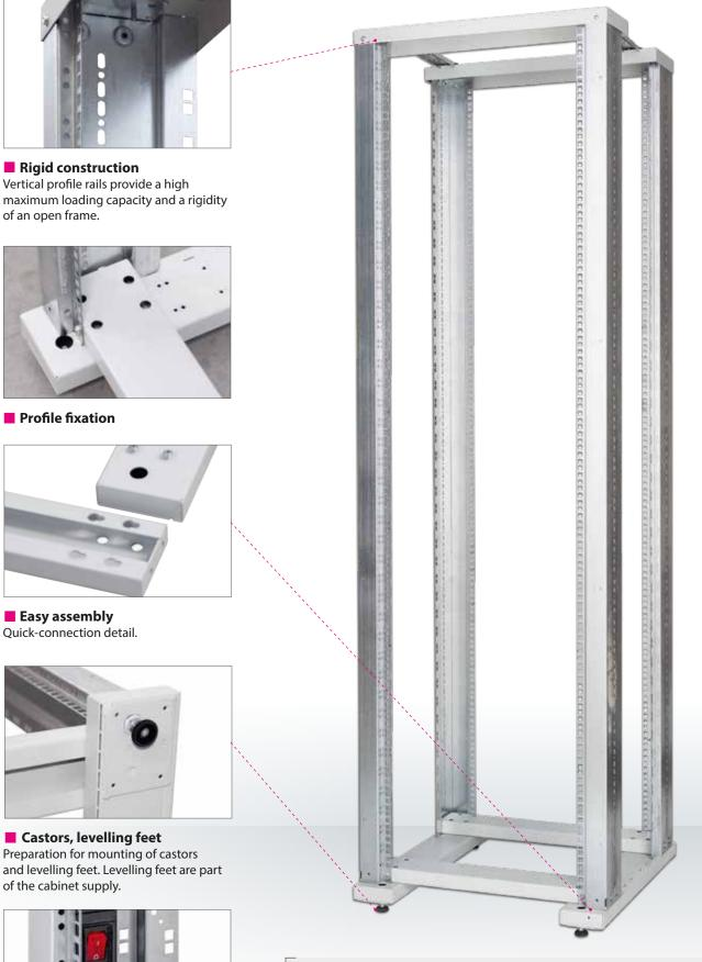
RSF-X open frame is supplied as double section only. Front and rear frame may be placed on the base in variety of distances to support installation of equipment with different depth.
